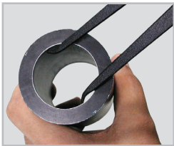
Inside Caliper: Used to measure the internal diameter of a cylinder
