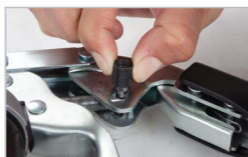
Pull button & slide to change mode between High Pressure/High Volume
