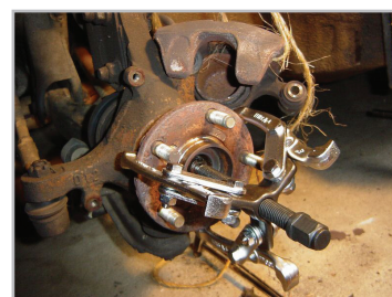
3 Jaw Puller used for removing tyre hub
